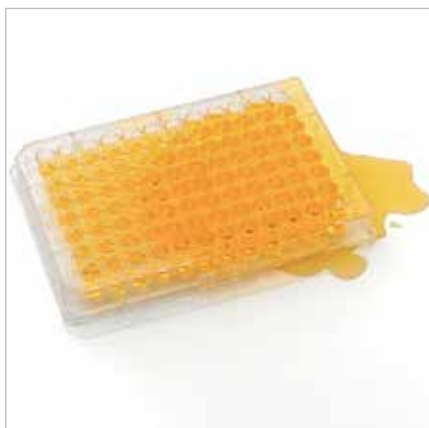
Spilling of plate caused by clogged needles
