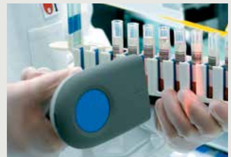
Barcode scanning before loading sample tubes onto the worktable
