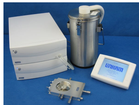
Geology System including LNP95 cooling system
