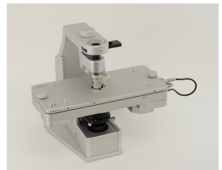
CSS450 stage open on the Linkam Imaging station. Sample image shows polymer flow using polarized light and phase contrast 10X objective.
