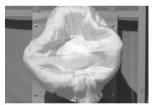
Airbag inflation can be recorded with more than 7000 frames/s at  $1k \times 1k$  resolution or with more than 5000 stereo images/s at  $1k \times 1k$  resolution (both images in one readout image with mirror set-up).
