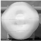
Different images of a highspeed sequence of an airbag inflation, which was recorded with two highspeed cameras. With the stereo setup it was possible to analyze the airbag inflation in three dimensions without any marker on the airbag.
