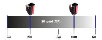
The graph shows the ISO 12232 values  $\rm s_{sat}$ ,  $\rm s_{40}$  and  $\rm s_{10}$  relative to the formerly used sensitivity values for negative film (examples give ASA 200 and ASA 1000) along a virtual sensitivity scale.
