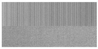
The top image shows the typical fixed pattern structures in the dark image of high speed CMOS image sensors, while the lower image shows less and more homogeneous noise in the dark image of a pco.dimax.
