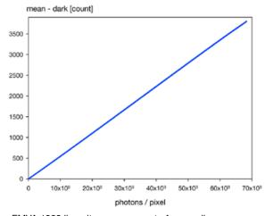
EMVA 1288 linearity measurement of a pco.dimax camera.
