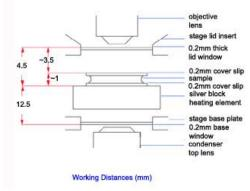
FTIR600 Horizontal — the diagram illustrates objective lens and condenser lens working distances.
